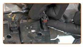
Remove the spark plug wire connectors from the spark plug wells. Use long round nose pliers.
