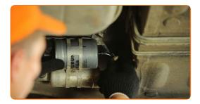
Tighten the fastening clamp of the fuel filter pipe. Use a flat screwdriver.
