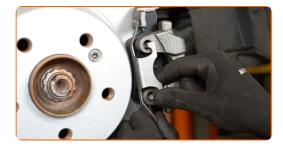
Connect the brake pads wear sensor.
