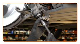
Replacement: brake pads – MERCEDES-BENZ S-Class Coupe (C215). Tip from AUTODOC:
