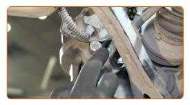
Install the brake caliper retaining spring.
