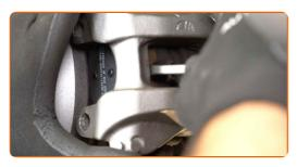
Remove the brake caliper.
