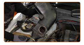
Disconnect the spark plug wires from the spark plugs.
