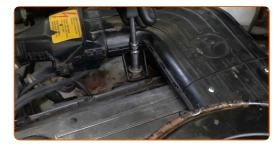
Connect the earth cable terminal to the battery.
