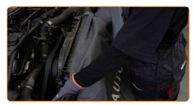
Disconnect the earth cable terminal from the battery. Use a combination spanner #10.
