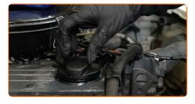
Tighten the oil filler cap.
