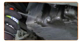
Screw in the new drainage plug and tighten it. Use a drive socket #13. Use a torque wrench. Tighten it to 27 Nm torque.
