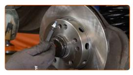
17 Remove the brake disc.
