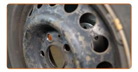
Tighten the screw of the wheel hub fastening nut. Use HEX No.H5. Use a torque wrench. Tighten it to 12 Nm torque.
