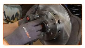
Remove the fastening bolt.
