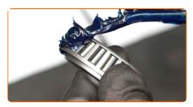
Reinstall the elements of the bearings in the wheel hub.
