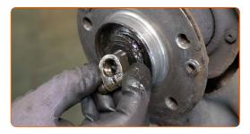
Remove the wheel hub together with the bearing. Use a universal puller.
