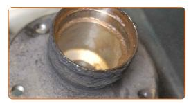
Install the outer rings of the new wheel bearings. Use a bush and bearing driver set.
