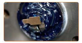
Install the hub bearing cap. Use a bush and bearing driver set. Use a hammer.
