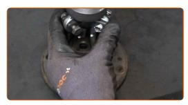
Clean the mounting seats of the wheel bearings. Use all-purpose cleaning spray.
