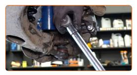
Secure the wiring to the strut.
