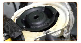
Screw on the fasteners of the upper strut mount.
