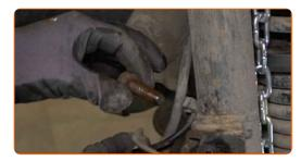
Detach the strut from the steering knuckle. Use a crowbar.
