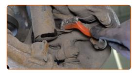
Unscrew the lower suspension strut fasteners. Use a combination spanner #19. Use a drive socket #19. Use a ratchet wrench.
