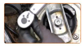
Tighten the fastener of the suspension strut piston rod. Use a special drive socket to remove the shock absorber # 19. Use HEX No.H6. Use a torque wrench. Tighten it to 60 Nm torque.
