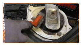
Clean the fastener of the suspension strut piston rod. Use a wire brush. Use WD-40 spray.
