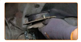
Clean the mounting seat of the suspension strut mount. Use a wire brush. Use all-purpose cleaning spray.
