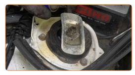
Loosen the fastener of the strut piston rod. Use a special drive socket to remove the shock absorber # 22. Use HEX No.H7. Use a ratchet wrench.
