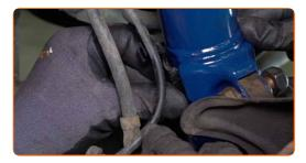
Screw on the fastener of the strut piston rod.
