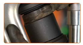
Clean the ball joint mounting seat. Use a wire brush. Use all-purpose cleaning spray.
