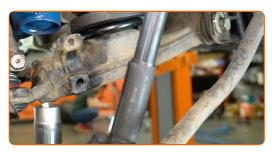
For tightening the fasteners correctly, you have to jack up the suspension components to their working position.
