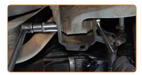
Unscrew the fastener connecting the ball joint to the steering knuckle. Use a combination spanner #19. Use a drive socket #19. Use a ratchet wrench.
