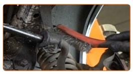
Unscrew the fasteners of the stabilizer bush brackets. Use a combination spanner #13. Use a drive socket #13. Use a ratchet wrench.
