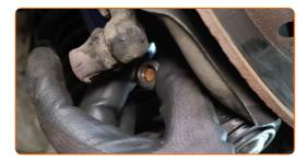
Tighten the fastener connecting the ball joint to the steering knuckle. Use a combination spanner #19. Use a drive socket #19. Use a torque wrench. Tighten it to 75 Nm torque.
