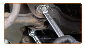
Tighten the rear fastener of the control arm. Use a combination spanner #22. Use a drive socket #22. Use a torque wrench. Tighten it to 120 Nm torque.
