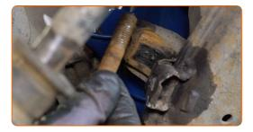
Disconnect the ball joint from the steering knuckle. Use a flat metal-working chisel. Use a hammer. Use a crowbar.
