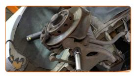
Install the coil spring compressor on the coil spring.
