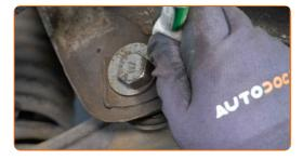
Unscrew the front fastener of the control arm. Use a combination spanner #22. Use a drive socket #22. Use a ratchet wrench.
