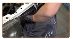
3 4 5 Unscrew the coolant reservoir cap.
