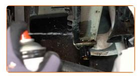
Unscrew the fan housing fasteners. Use a combination spanner #10. Use a drive socket #10. Use a ratchet wrench.
