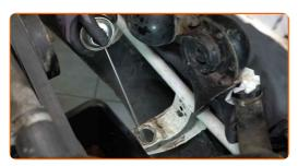
Fit the engine cooling radiator mounting pads.
