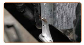
Screw in the fasteners of the fan housing. Use a combination spanner #10. Use a drive socket #10. Use a ratchet wrench.
