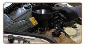
Pour coolant in the coolant reservoir.
