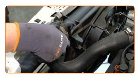
Tighten the clamp of the upper coolant hose. Use a drive socket #7. Use a ratchet wrench.
