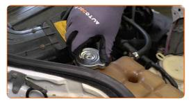
Screw on the coolant reservoir cap.
