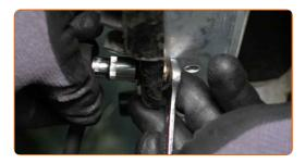
29 Attach the lower coolant pipe.
