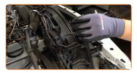
Remove the upper engine radiator clips. Use long nose pliers.
