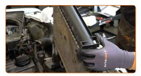
Remove the engine cooling radiator mounting pads.
