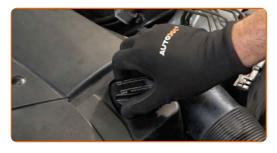
33 Tighten the oil filler cap.
