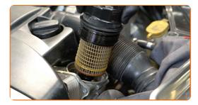
Replacement: engine oil and filter – MERCEDES-BENZ M-Class (W164) V6. AUTODOC recommends:
