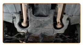
Tighten the fasteners of the oil pan lower cover. Use a drive socket #8. Use a ratchet wrench.
