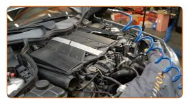
Remove the air filter housing.
