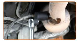
11 Remove the oxygen sensor.
