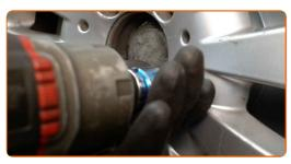
Lower the car and working in a cross order, tighten the wheel bolts. Use wheel impact socket #17. Use a torque wrench. Tighten it to 130 Nm torque.
