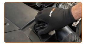
33 Tighten the oil filler cap.
