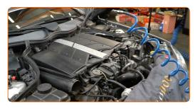
Remove the air filter housing.
