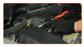
Remove the crankcase ventilation hose. Use a flat screwdriver.
