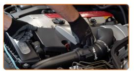
Replacement: engine oil and filter – MERCEDES-BENZ G-Class Off-Road (W463). Tip from AUTODOC:
