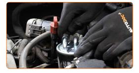
Tighten the fastening clamp of the fuel filter pipe. Use a drive socket #7. Use a ratchet wrench.
