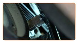
Rotate the crankshaft several times to check whether the new V-ribbed belt is working correctly. Use a drive socket #27. Use a ratchet wrench.
