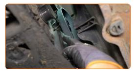
Pull aside the V-ribbed belt tensioner pulley. Use 12-point socket No.17. Use a ratchet wrench.
