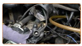
Remove the high tension cable from the ignition coil cover. Use a crowbar.
