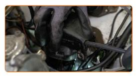
21 Install the high tension cable bracket.
