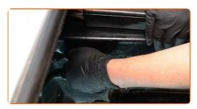
Remove the bulb holder together with the bulbs.
