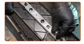
Treat the bulb holder terminals on the cover. Use dielectric grease.
