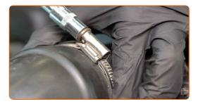
17 Treat the mass air flow sensor connector. Use dielectric grease.
