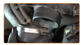
Undo the fastening screws of the air filter cover. Use a drive socket #E11. Use a ratchet wrench.
