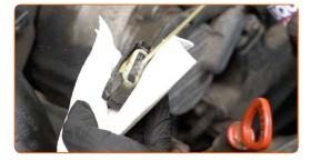
Attach the mass air flow sensor connector.
