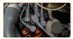
Disconnect the spark plug wires from the spark plugs.
