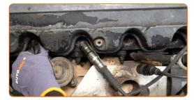
Disconnect the high tension cables from the ignition distributor.
