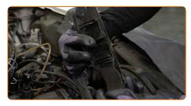
Make marks to indicate the order of installation of the spark plug wires.
