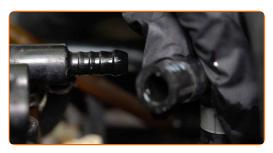
Prime the fuel system manually. Use a bulb hand fuel pump.
