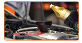
Unscrew the oil filler plug. Insert the funnel.
