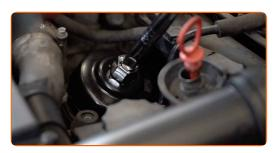
Screw the new filter into its place.
