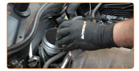
Release the mass air flow sensor retaining clips. Use a crowbar.
