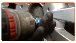
Lower the car and working in a cross order, tighten the wheel bolts. Use wheel impact socket #17. Use a torque wrench. Tighten it to 130 Nm torque.
