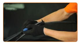
Remove the blade from the wiper arm.
