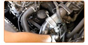
Pull aside the V-ribbed belt tensioner pulley. Use Torx T55. Use a ratchet wrench.
