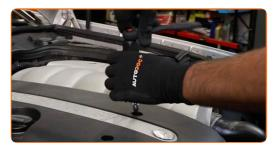
Unscrew the fasteners of the back section of the engine cover. Use a drive socket #10. Use a ratchet wrench.
