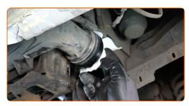
Clean the mounting seats of the intercooler hose. Use all-purpose cleaning spray.
