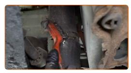
Unscrew the intercooler pipe clamp. Use a drive socket #7. Use a ratchet wrench.
