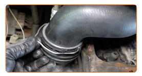
Replacement: intercooler hose – MERCEDES-BENZ E-Class T-modell (S210).
