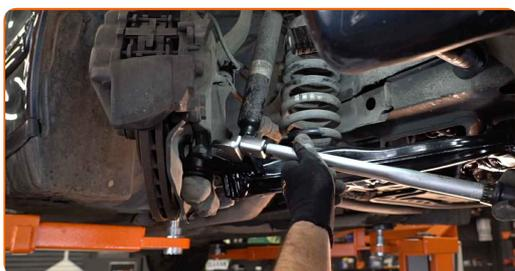
**50** install the rod fastening to the stabilizer and tighten it. Use Torx T50. Use a torque wrench. Tighten it to 45 nm torque.
