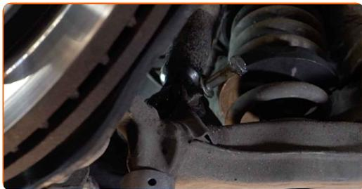
**19** Unscrew the front arm fastener. Use a combination spanner #22 (2 pieces).
