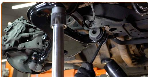
**35** Install the control arm fasteners. Use a rubber mallet.
