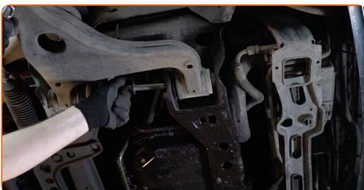
**25** Unscrew the fastener connecting the ball joint to the suspension control arm. Use a combination spanner #22.
