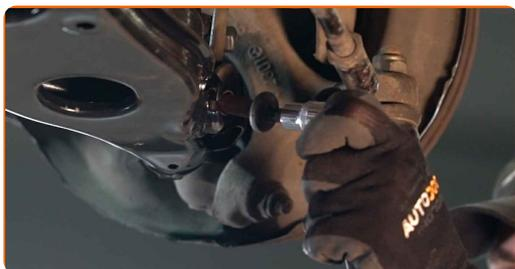
**49** Tighten the ball joint fastener. Use a combination spanner #22. Use a torque wrench. Tighten it to 80 nm torque.
