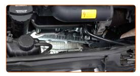
Unscrew the ignition coil bracket. Use a drive socket #E11. Use a ratchet wrench.
