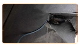
Screw in the fasteners of the side trim panel. Use a Phillips screwdriver.
