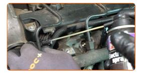
Attach the glow plug wiring connectors. Use needle nose pliers.
