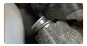
Detach the glow plug wiring connectors. Use needle nose pliers.
