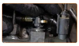
Tighten the fuel hose fastener. Use a drive socket #E11. Use a torque wrench. Tighten it to 8 nm torque.
