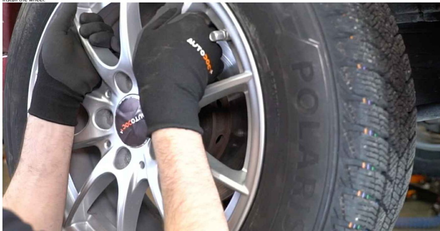
Replacement: coil springs - MERCEDES-BENZ E-Class T-modell (S124). AUTODOC recommends: • To avoid injury, hold up the wheel when screwing in the fastening bolts.
