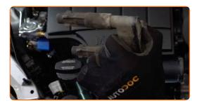
6 Unscrew the spark plugs. Use the spark plug socket #16. Use a ratchet wrench.
