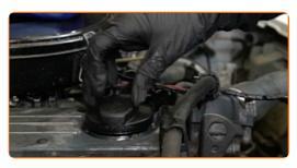
Tighten the oil filler cap.
