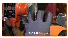
Remove the retaining spring of the brake pads.
