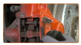
Remove the brake pad guide pins. Use a pin punch. Use a hammer.
