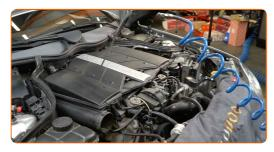
Remove the air filter housing.
