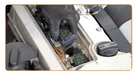
Treat the ignition coil tip. Use high-temperature grease. Use a flat screwdriver.
