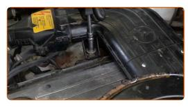
Connect the earth cable terminal to the battery.
