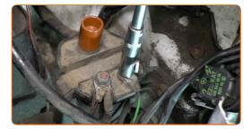
Disconnect the terminals from the ignition coil.
