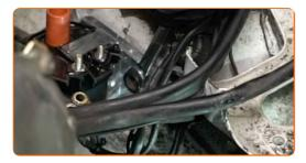
Connect the terminals to the ignition coil.
