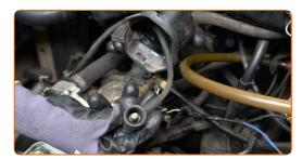
Unscrew the fasteners of the ignition coil terminals. Use a drive socket #10. Use a ratchet wrench.
