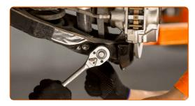
Unscrew the fastener connecting the stabilizer link to the stabilizer bar. Use a combination spanner #17. Use a combination spanner #19.
