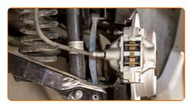
Tighten the fastener connecting the stabilizer link to the stabilizer bar. Use a combination spanner #17. Use a combination spanner #19. Use a torque wrench. Tighten it to 30 Nm torque.
