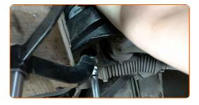
Remove the support from under the engine.
