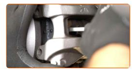
14 Remove the brake caliper.
