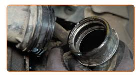
Cover the air hoses with microfibre cloths to prevent dirt from entering the system.
