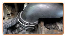
Replacement: intercooler hose – MERCEDES-BENZ E-Class Platform / Chassis (VF210). Professionals recommend:
