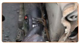
Remove the lower clip of the intercooler hose. Use a crowbar.
