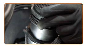
Install a new mass air flow sensor. Make sure you hear a click indicating that it is locked in place.
