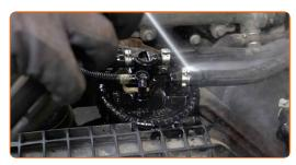
Remove the retaining clip that secures the fuel filter pipe.
