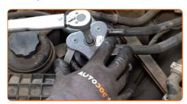
Connect the pipe to the fuel filter.
