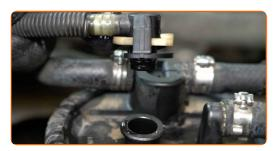
6 Unscrew the fasteners of the fuel filter housing cover. Use a universal puller.
