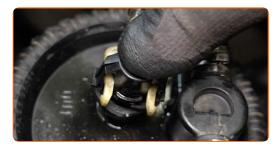
Secure the fuel filter pipe with the retaining clip.
