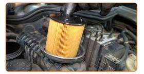
Pump the fuel out of the fuel filter housing. Use an automotive fluid syringe.
