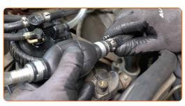
Replacement: fuel filter – MERCEDES-BENZ E-Class Platform / Chassis (VF210). Professionals recommend:
