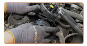
14 Install and tighten the fuel filter housing cap.
