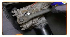
Unscrew the fastener connecting the linkage to the wiper motor shaft. Use a drive socket #13. Use a ratchet wrench.
