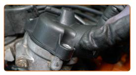
Replacement: engine thermostat – MERCEDES-BENZ E-Class Coupe (C124). Tip from AUTODOC experts:
